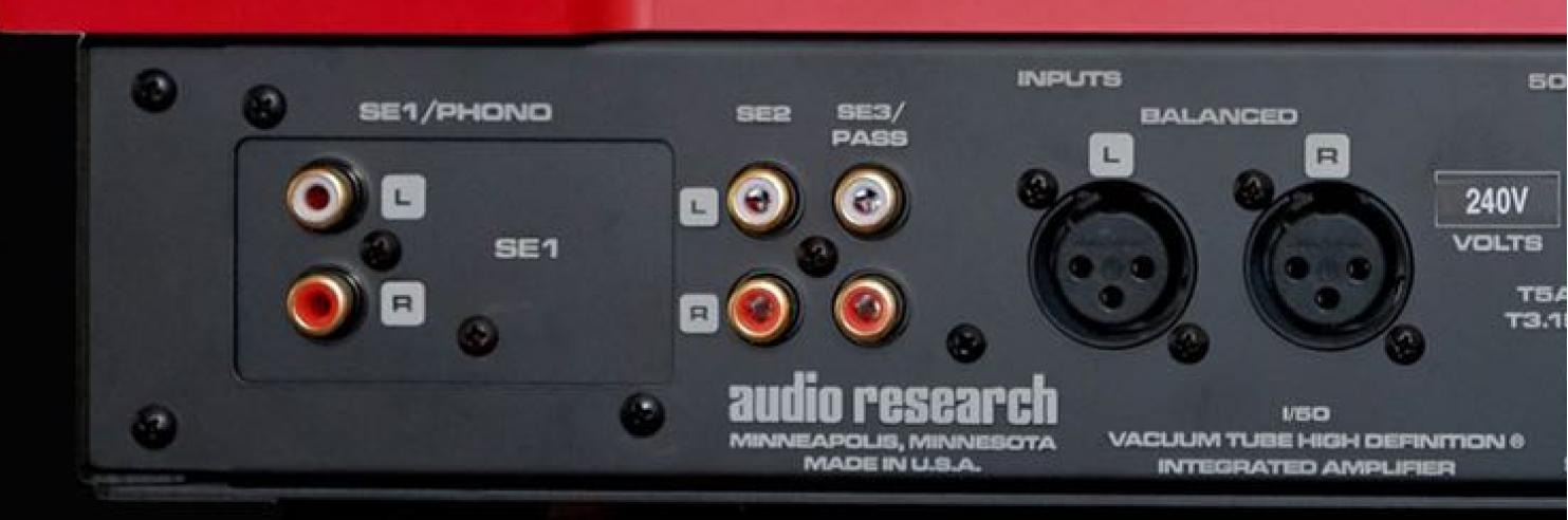
On the rear panel, we find three RCA inputs (No. 1 serves the Phono module when installed), No. 3 allows bypass when selected plus an XLR input. There is also a slot for the future DAC, which is already equipped with the appropriate inputs and outputs.
